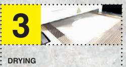
Allow the printed and powdered film to cure in the dryer. The powder is melting and build a protective layer over the printing.
