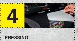
At least press the dried film onto the garment with a heat press, wait a few seconds until the film is cool and remove it.
