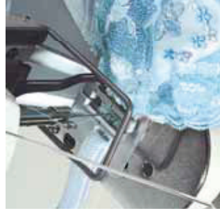
F type (Attaching the shoulder straps to brassier) * Presser foot for vertical barracking is supplied with the unit as an accessory.
