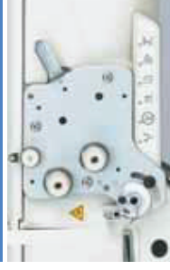
① Alternating vertical movement of the walking foot and presser foot changeover switch / ② Automatic reverse / ③ Sewing prohibition changeover switch / ④ Needle up/down switch / ⑤ Needle thread clasp switch (ST7) / ⑥ Tension disk No. 1 operation switch / ⑥ Needle thread clasp switch (for the thread remaining type)
